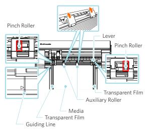
\* Align the left edge of the transparent film against the Guiding Line on the front panel.
