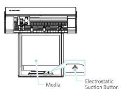
3 Check that the lamp above the electrostatic suction button (white) turns on and that it is functioning properly.
