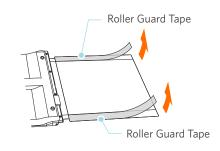
Affix the replacement roller guard tape along the white lines on both sides.
